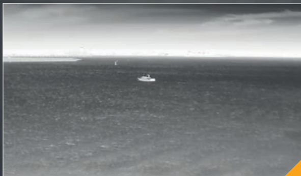
FLIR Vision: Thermal imaging is immune to visible light and glare. Not only can we clearly see the police boat, we can also see the buoy and jetty astern of it.
