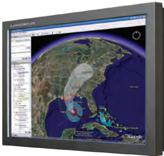
42" Model WFP42W2 Native Resolution 1920 x 1080 (FHD) Bright 700 nits with LED BL Video Inputs: VGA, DVI-D Bonded 6mm AR Window Optional IR Touch System VESA 100/200/400mm Mount Designed To Meet MIL-STD 901D Grade A
