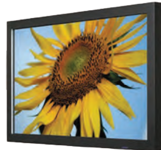
55" Model CFP55W1 Native Resolution 1920 x 1080 (FHD) Bright 700 nits with LED BL Video Inputs: VGA, DVI Bonded 6mm AR Window Optional IR Touch System VESA 100/200/400mm Mount Designed To Meet MIL-STD 901D Grade A
